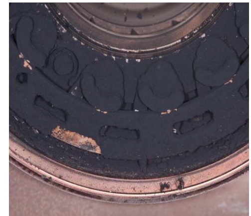
VTG Soot Test – STILL FUNCTIONAL
