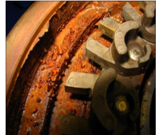
VTG Corrosion Test – STILL FUNCTIONAL
